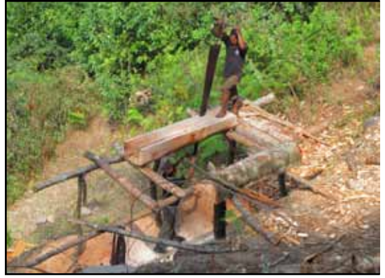
Day 8. Building timber is still cut by hand. Here a long saw is operated by two cutters. The "top dog" has to pull the 3 kg saw up but the "underdog" gets covered in sawdust.
